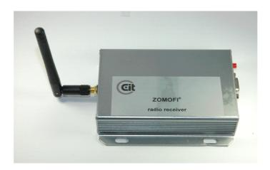
CITSens Bio ZOMOFI® receives data from CITSens Bio Beamer which is connected to the CITSens Bio sensor Glucose, Lactate and Glutamate. CITSens Bio ZOMOFI® can receive measurement data from up to 1000 sensors and transfers them to the PC by means of LAN.
