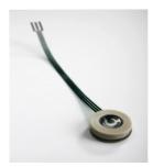
Regardless the types of reactors you are using, **CITSens Bio** is suitable for all standard disposable reactors such as t-flask, roller flasks, Erlenmeyer and bag-reactor. The sensor is built into the corresponding original cap and delivered to the customer gamma-sterilized and ready for use.
